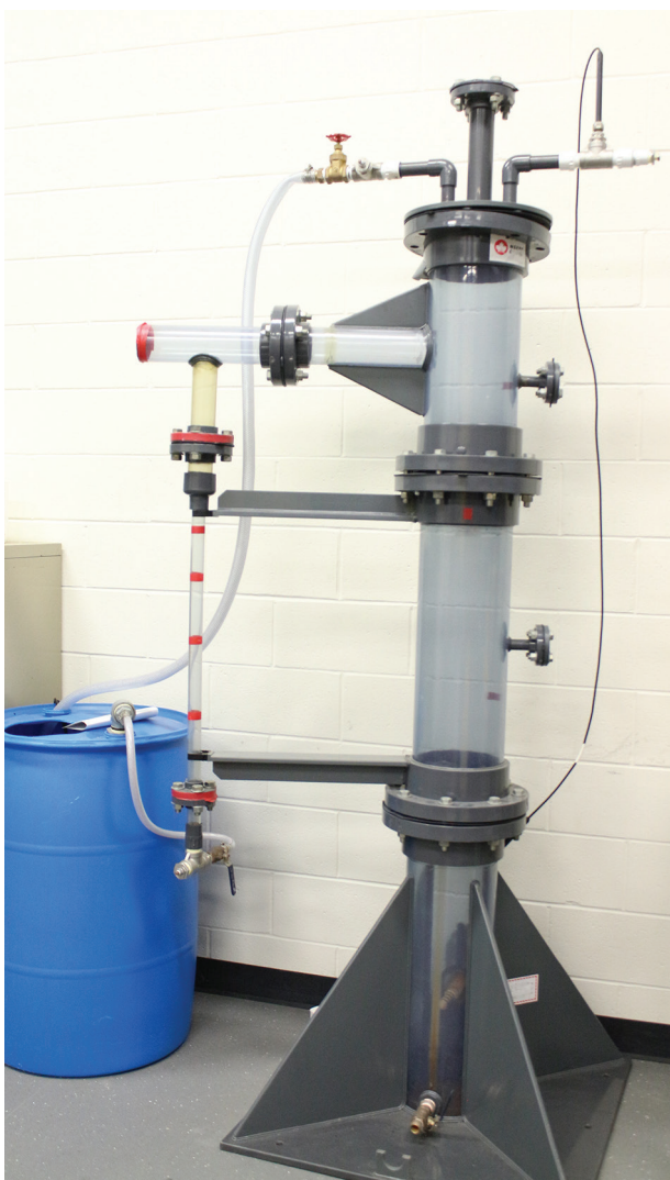
This Multiphase Flow Column was a key part of Dr. Jianu's previous work, where she would spend days on end counting the bubbles to get her conclusion.
